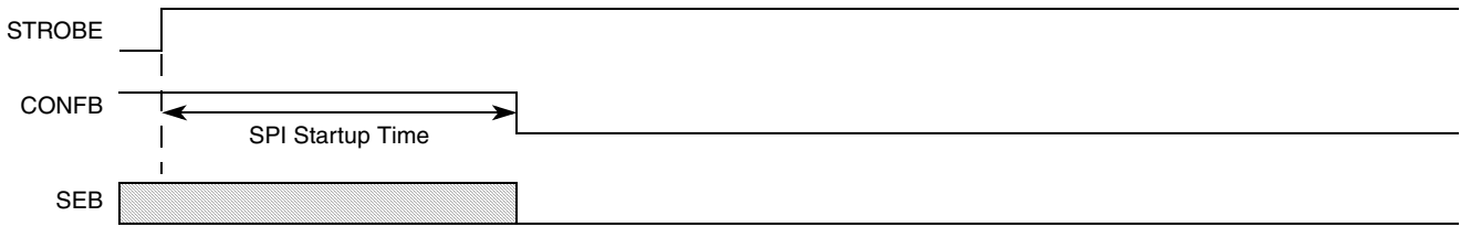
Figure 28. First Valid Sequence from Standby/LVD Mode to Configuration Mode
